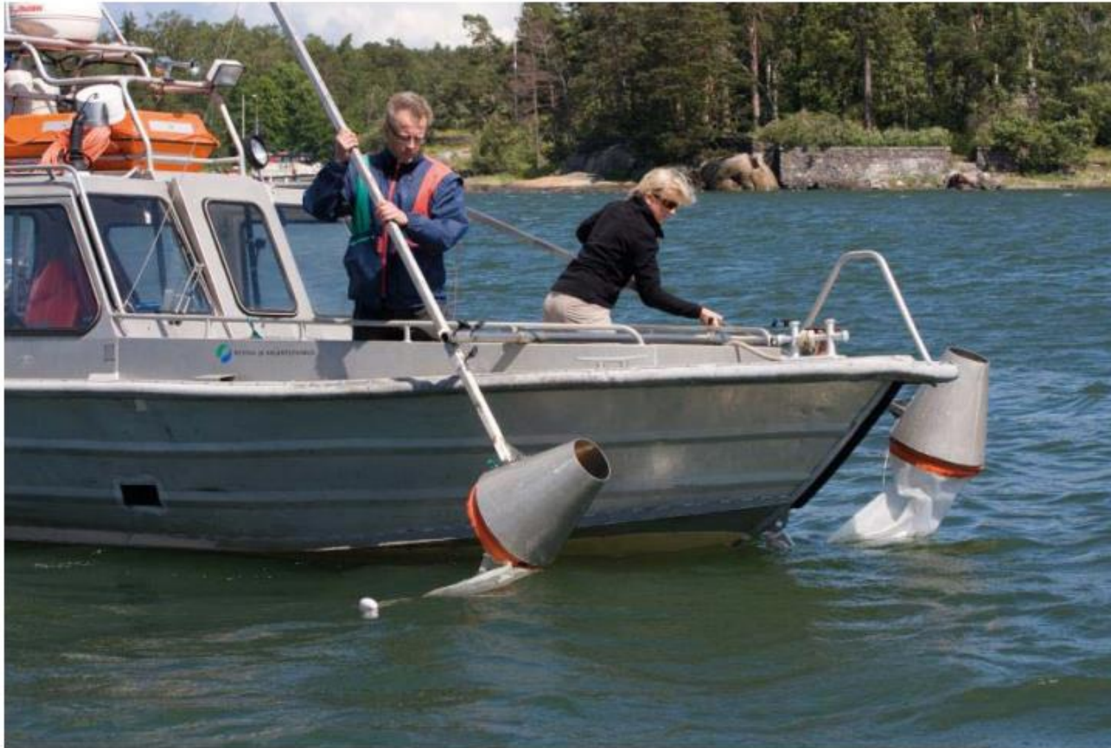
Figure 1. Gulf Olympia paired ichthyoplankton samplers are mounted parallel to each other at the bow of the boat, allowing for simultaneous sampling of different depths (0.25 – 2 m). The nosecones are lifted out of the water for collection of the samples and during transport between sampling sites (photo: Lari Veneranta, Luke)
